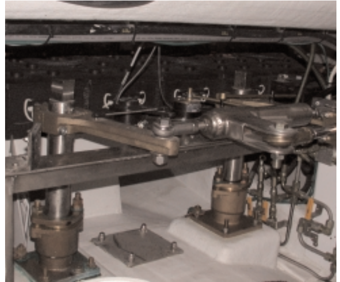
Close-up views of the steering mechanism. Because the two rudders move as one, the controls are stationary in relation to each other. Hydraulic rams are attached to the steering posts.
