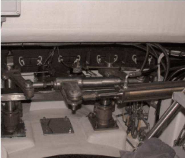
Close-up views of the steering mechanism. Because the two rudders move as one, the controls are stationary in relation to each other. Hydraulic rams are attached to the steering posts.
